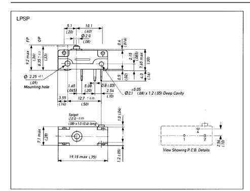
The Low Profile series is an innovative approach to the increasing use of printed circuit boards as carriers of electrical-electronic switching units.
